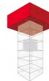
Machine room in the ordinary elevator
